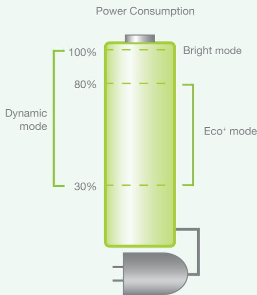
Dynamically adjusts the brightness and power consumption
